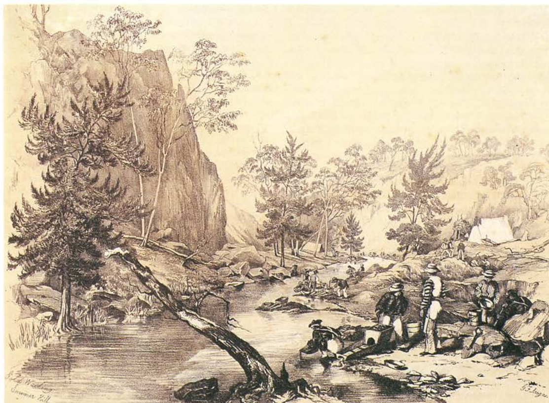
Goldwashing, Summer Hill Creek, 1851, a lithograph by George French Angas, illustrates the labour-intensive nature of alluvial goldmining on the Ophir goldfield in NSW. All the equipment is hand operated, and large numbers of diggers are ranged along the creek on small claims.
